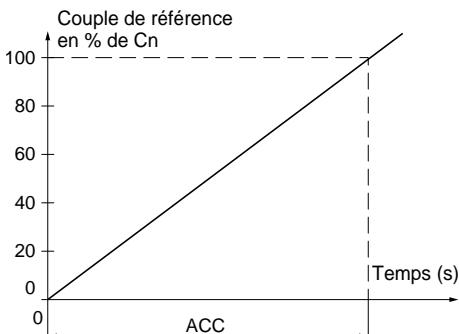
A graph illustrating the torque ramp during acceleration. The vertical axis is labeled "Couple de référence en % de Cn" (Torque reference in % of nominal torque) and ranges from 0 to 100. The horizontal axis is labeled "Temps (s)" (Time in seconds) and has a point labeled "ACC". A straight line starts at the origin (0,0) and rises linearly to the 100% mark on the y-axis, corresponding to a specific time value on the x-axis. |       |               |               |
