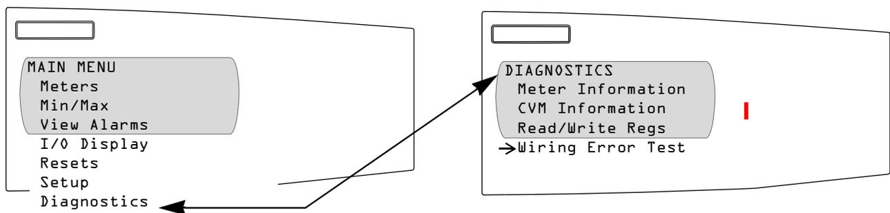
**Figure 3–10: Wiring Error Test option on the Diagnostics menu.**
