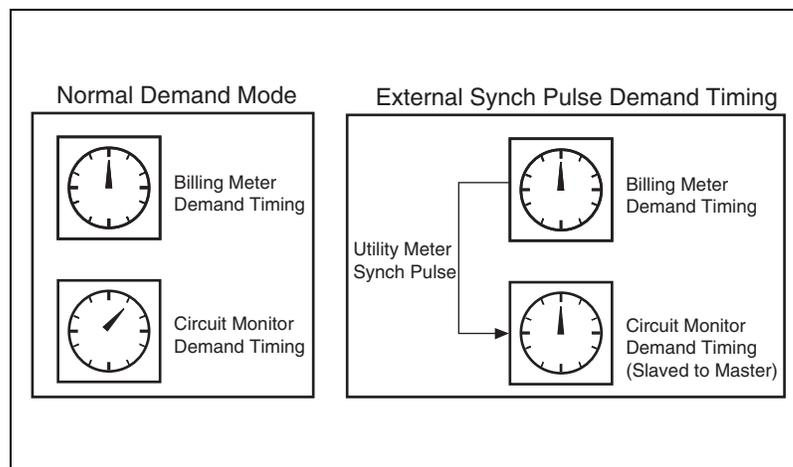
Figure 5–1: Demand synch pulse timing
