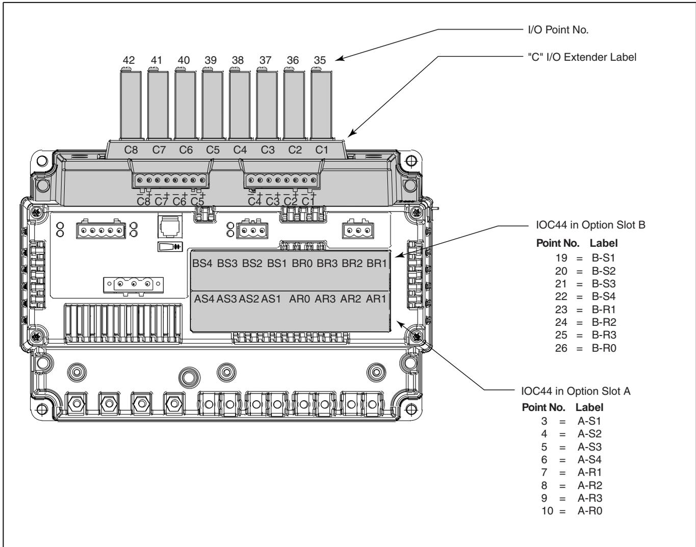
Figure B-2: Identifying I/Os for the command interface
