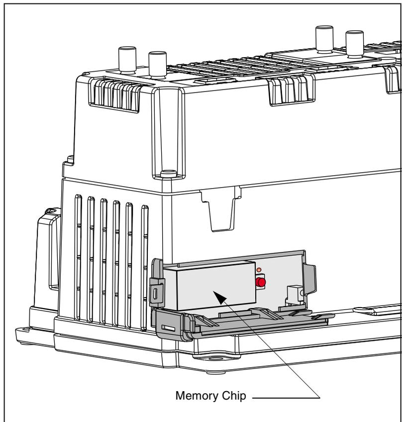
Figure 10–1: Memory chip location in the circuit monitor
