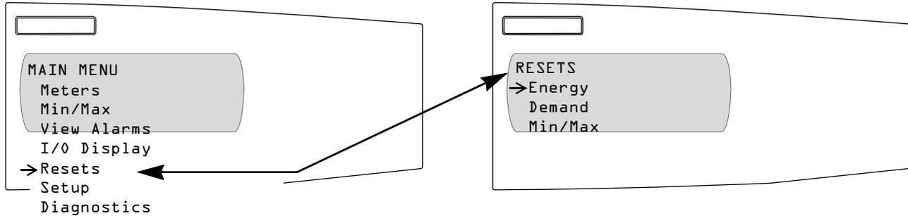
Figure 3–6: Performing resets from the Reset menu
