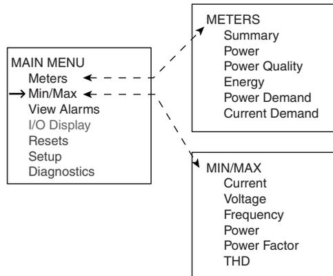
**Figure 3–7: Viewing metered data on the Meters and Min/Max menus**
