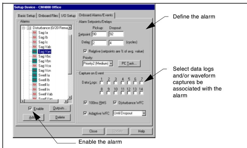
Figure 9-4: Onboard Alarms/Events tab
