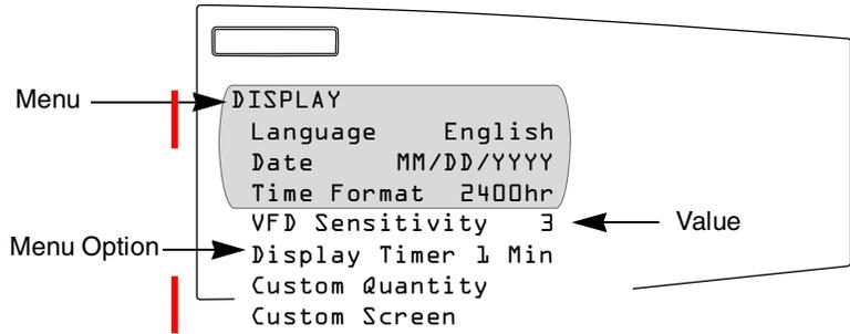
Figure 3–3: Parts of a menu
