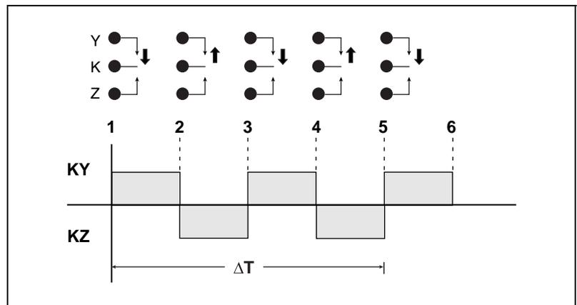
Figure 5–4: Three-wire pulse train
