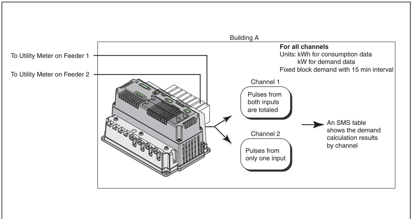
Figure 4–6: Channel pulse metering example
