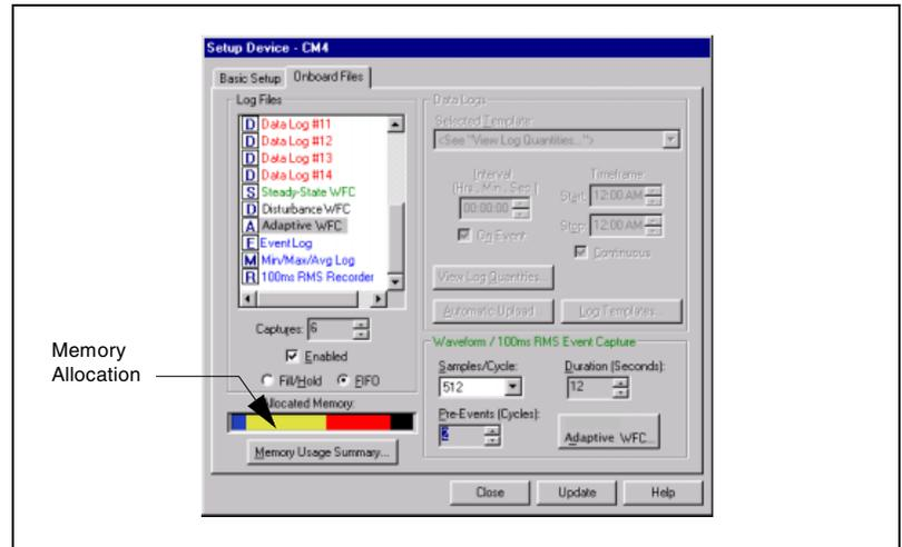
Figure 7–2: Memory allocation in SMS
