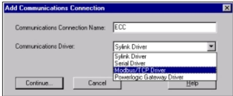
**Figure 5–1: Select MODBUS/TCP Driver in the Add Communications Connection dialog box**
