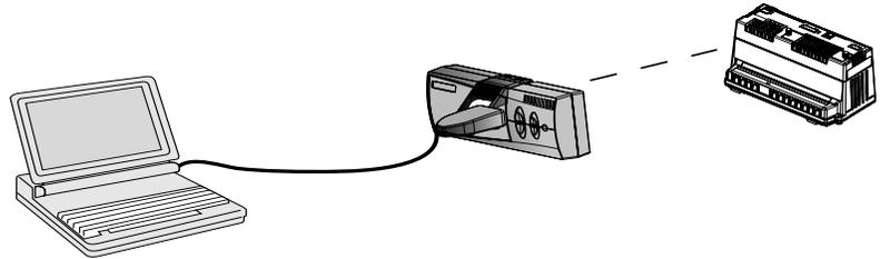
**Figure 6–3: Optical Communications Interface (OCIVF)**
