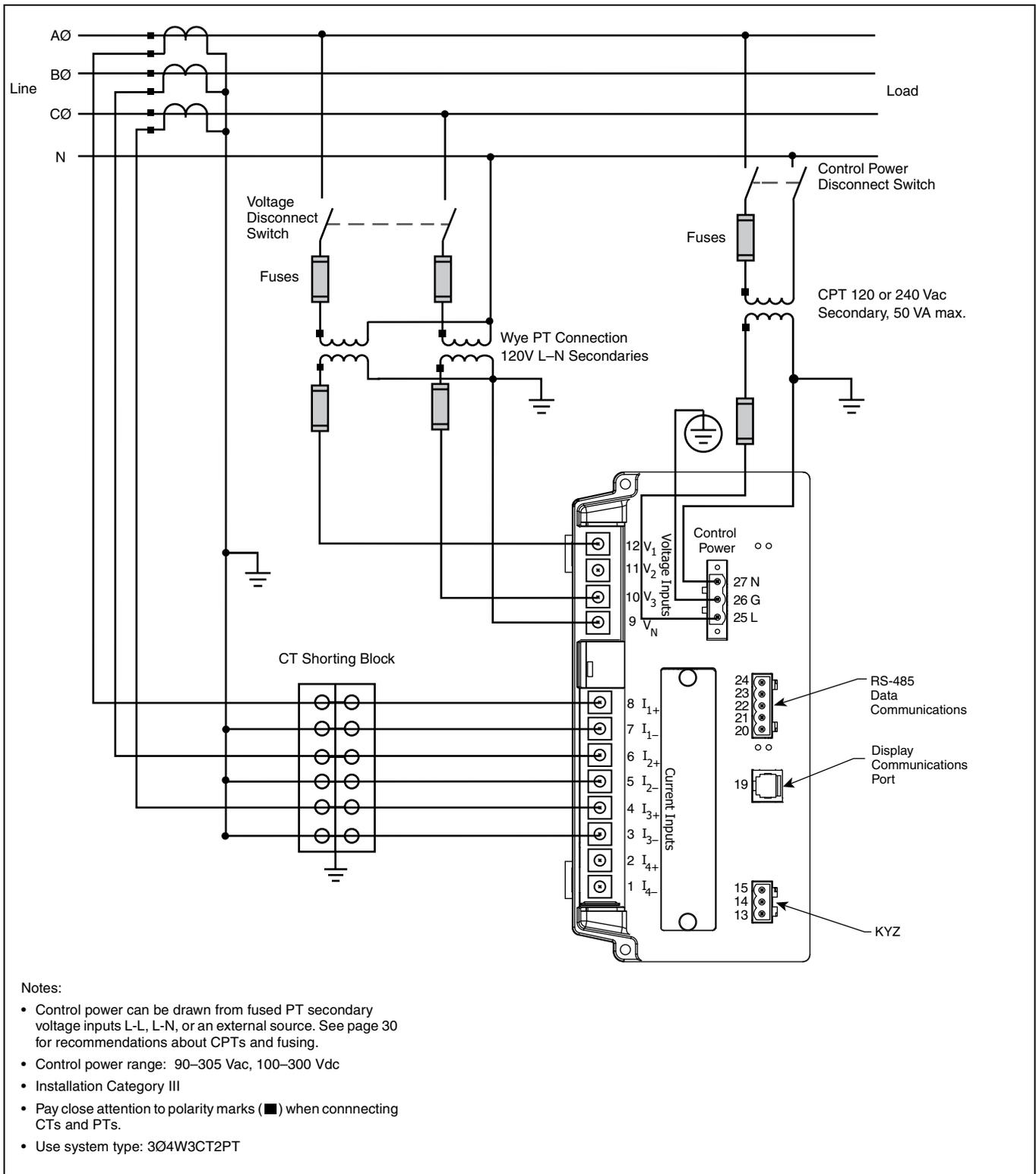
Figure 5–11: 3-Phase, 4-Wire Wye with 3CTs and 2 PTs (calculated neutral).
