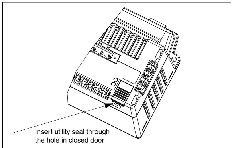
**Figure 4–14: Securing the access door**
