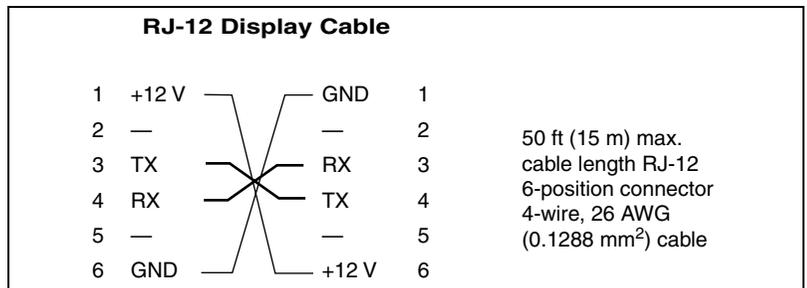
Figure 4-10: RJ-12 display cable pinout
