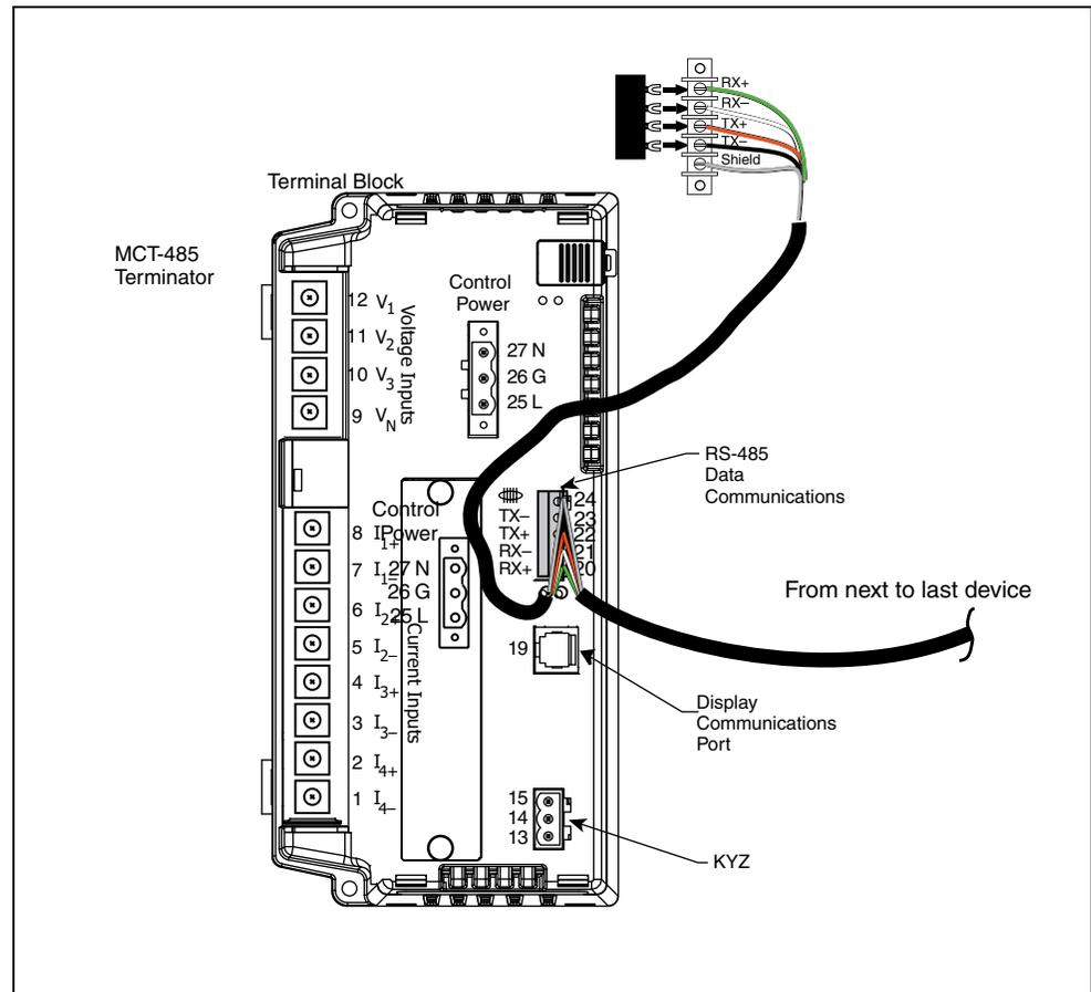
Figure 6–9: Terminating the circuit monitor using the MCT-485 terminator and a terminal block
