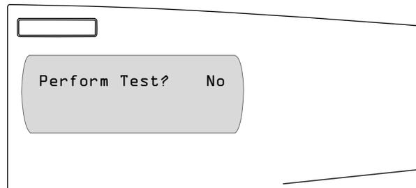
5. Select "Yes" to perform the test by pressing the up arrow button and then pressing the enter button.
