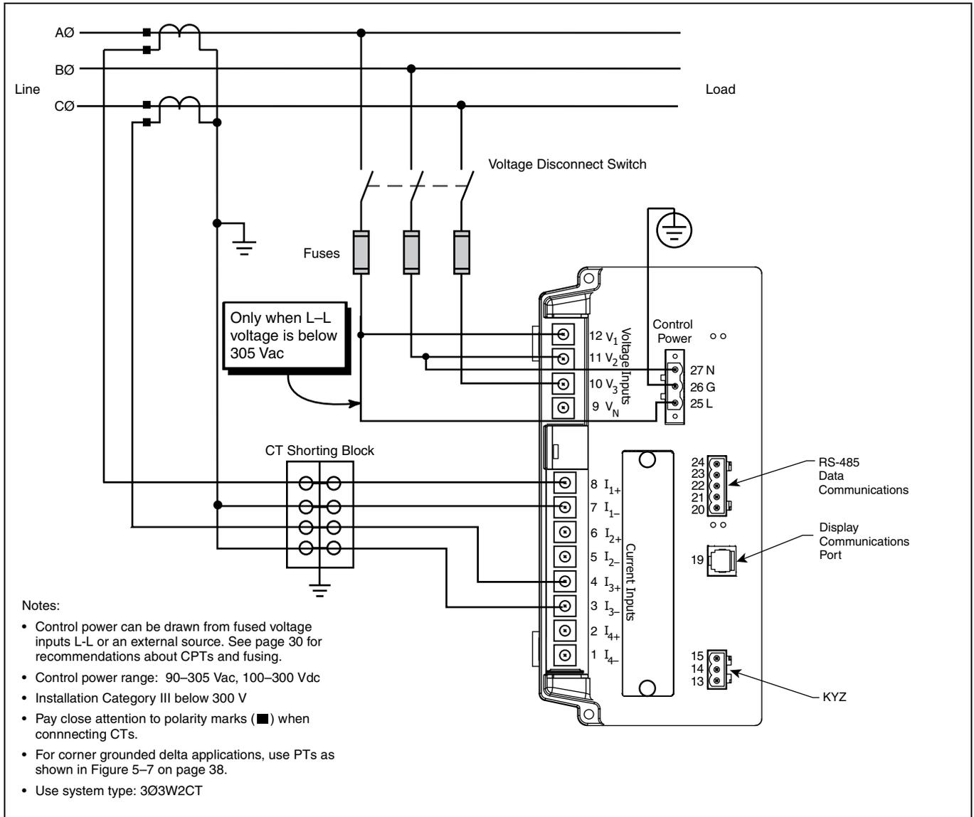
Figure 5–4: 3-Phase, 3-Wire Delta Direct Voltage Connection with 2 CTs
