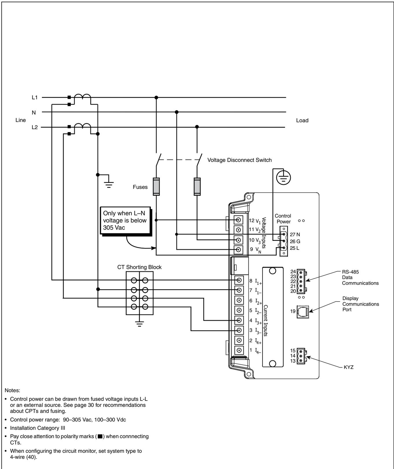
Figure 5–13: 1-Phase, 3-Wire Direct Voltage Connection with 2 CTs
