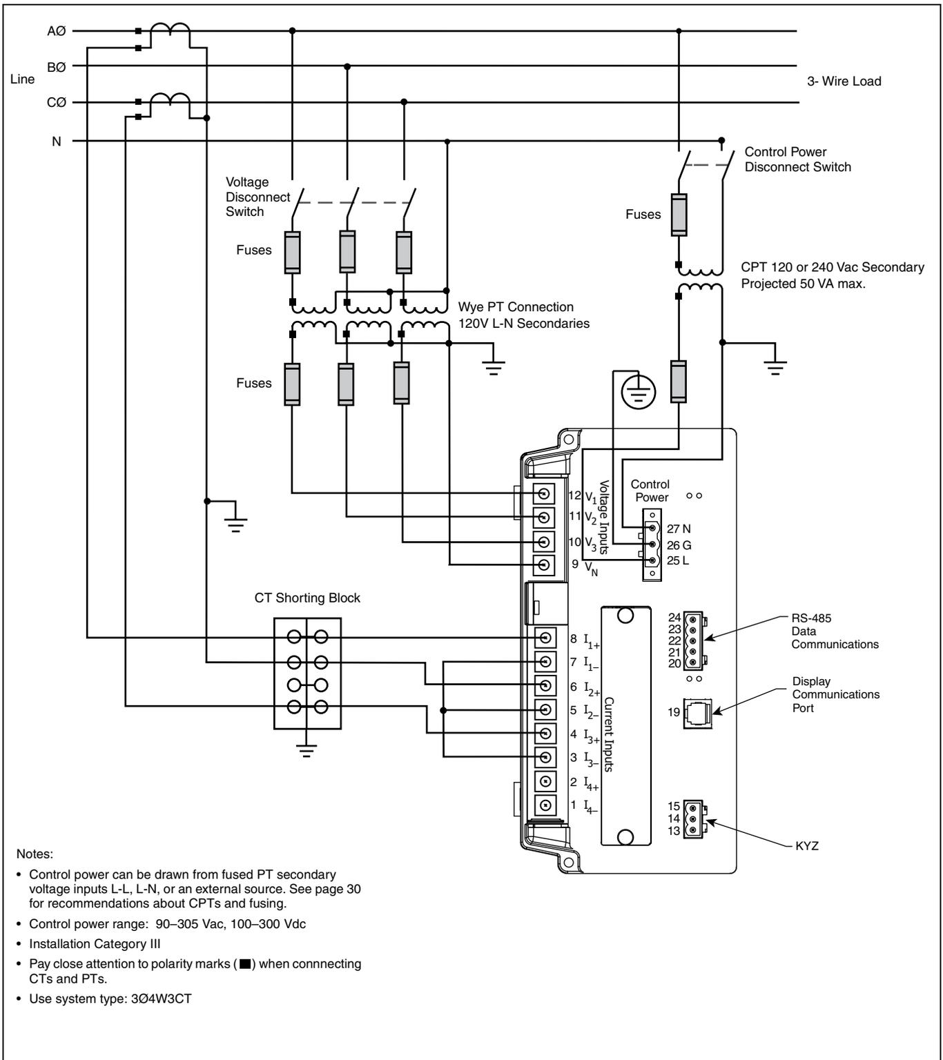
Figure 5–10: 3-Phase, 3-Wire Wye, 3-Wire Balanced Load with 3 PTs and 2 CTs
