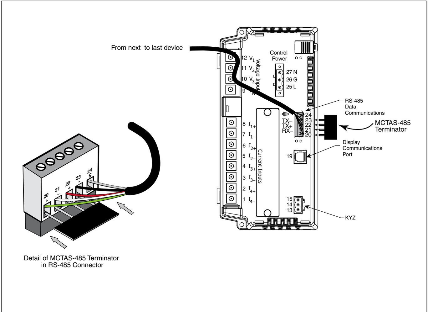
**Figure 6–8: Terminating the circuit monitor using the MCTAS-485 terminator**
