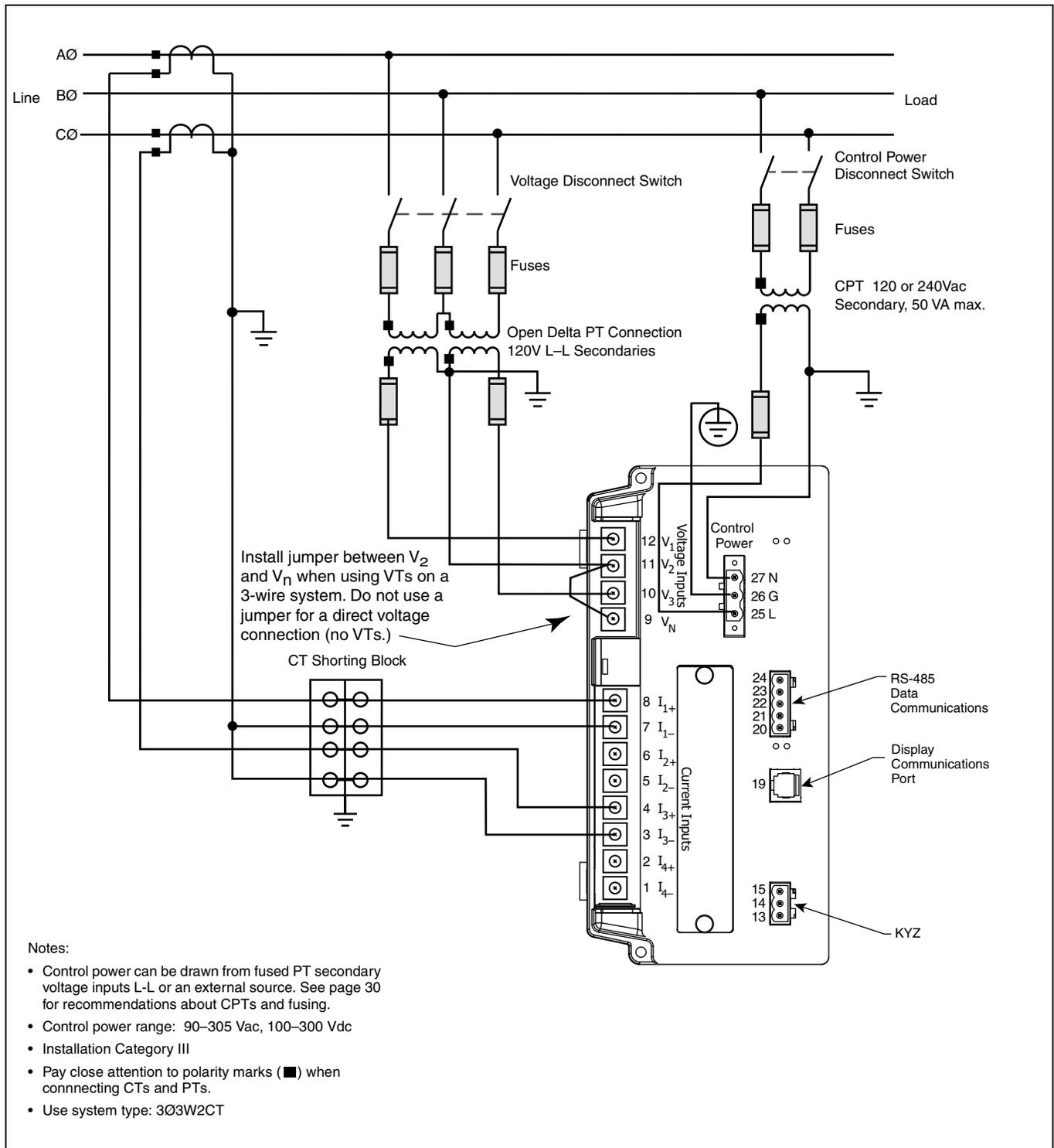
Figure 5–5: 3-Phase, 3-Wire Delta Connection with 2 PTs and 2 CTs
