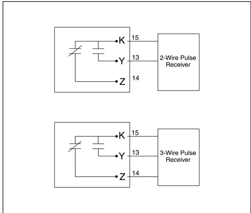
**Figure 5–19: KYZ pulse output wiring diagram.**
