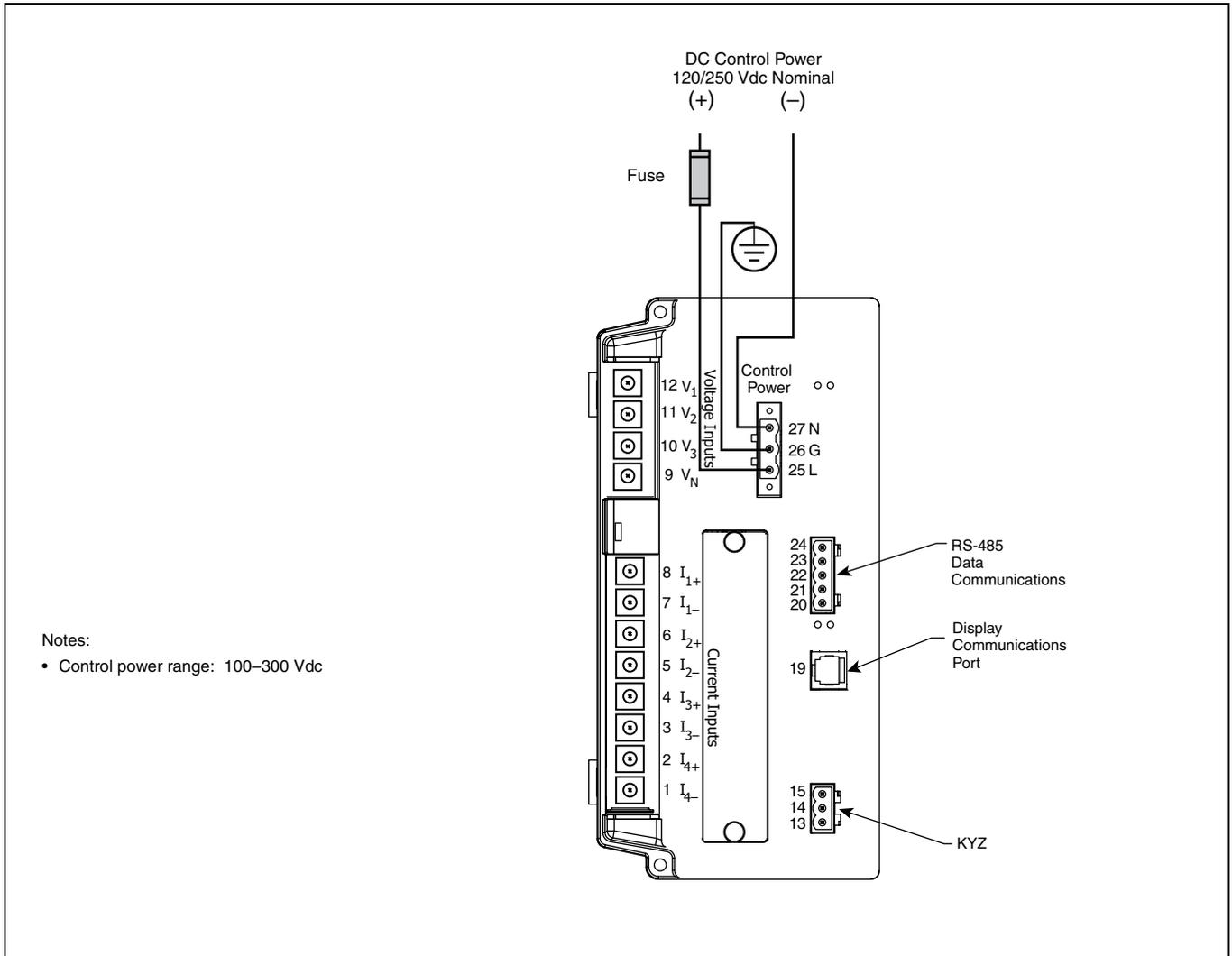
Figure 5–14: DC Control Power Wiring
