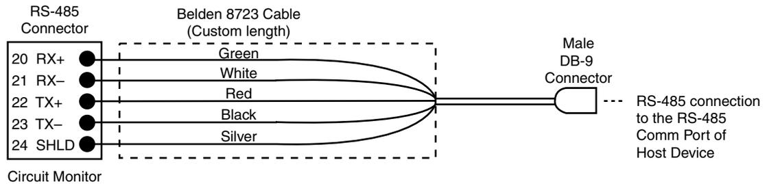
**Figure 6–7: Typical procedure for connecting the first device on the daisy chain**
