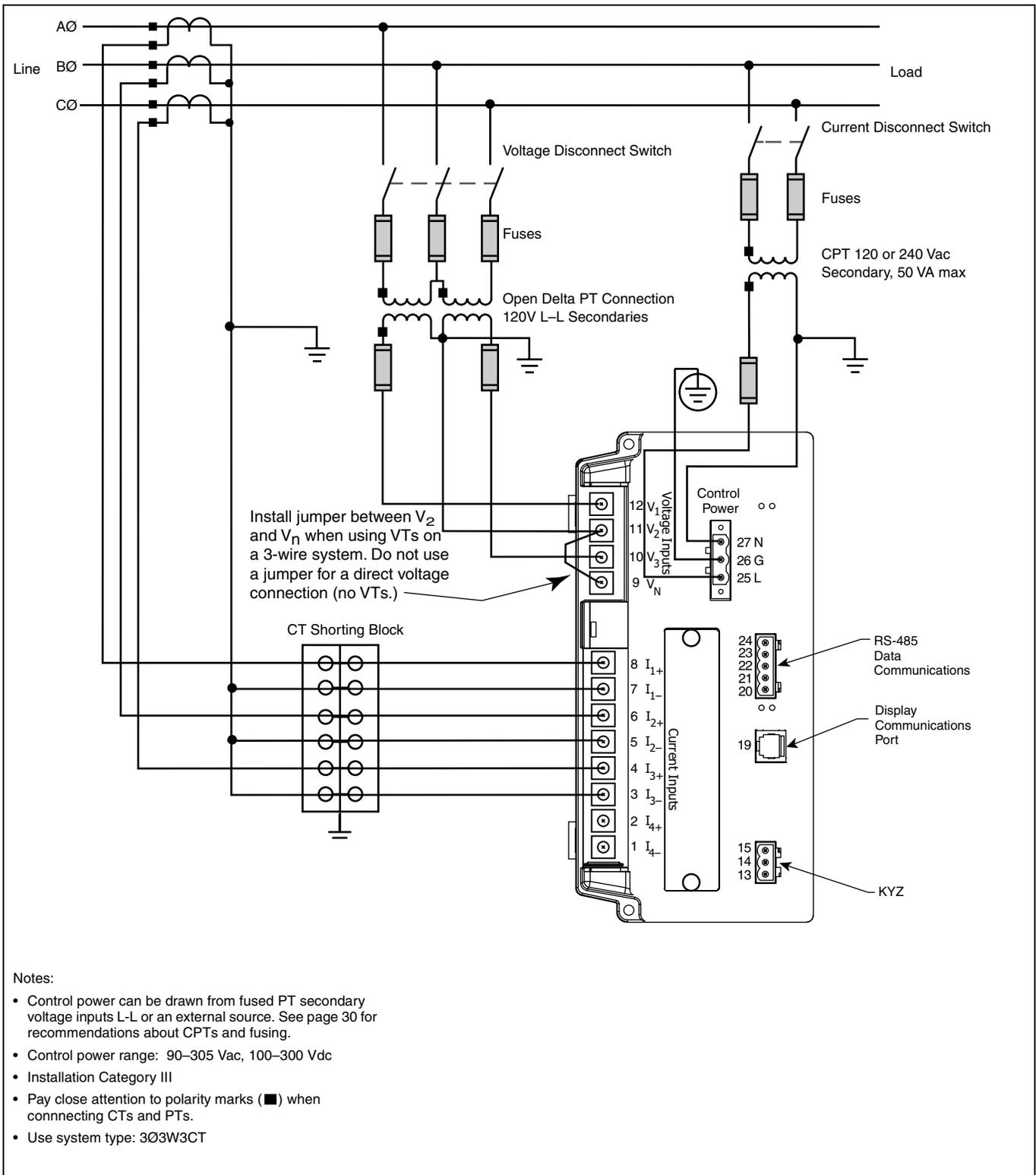
Figure 5-6: 3-Phase, 3-Wire Delta Connection with 2 PTs and 3 CTs
