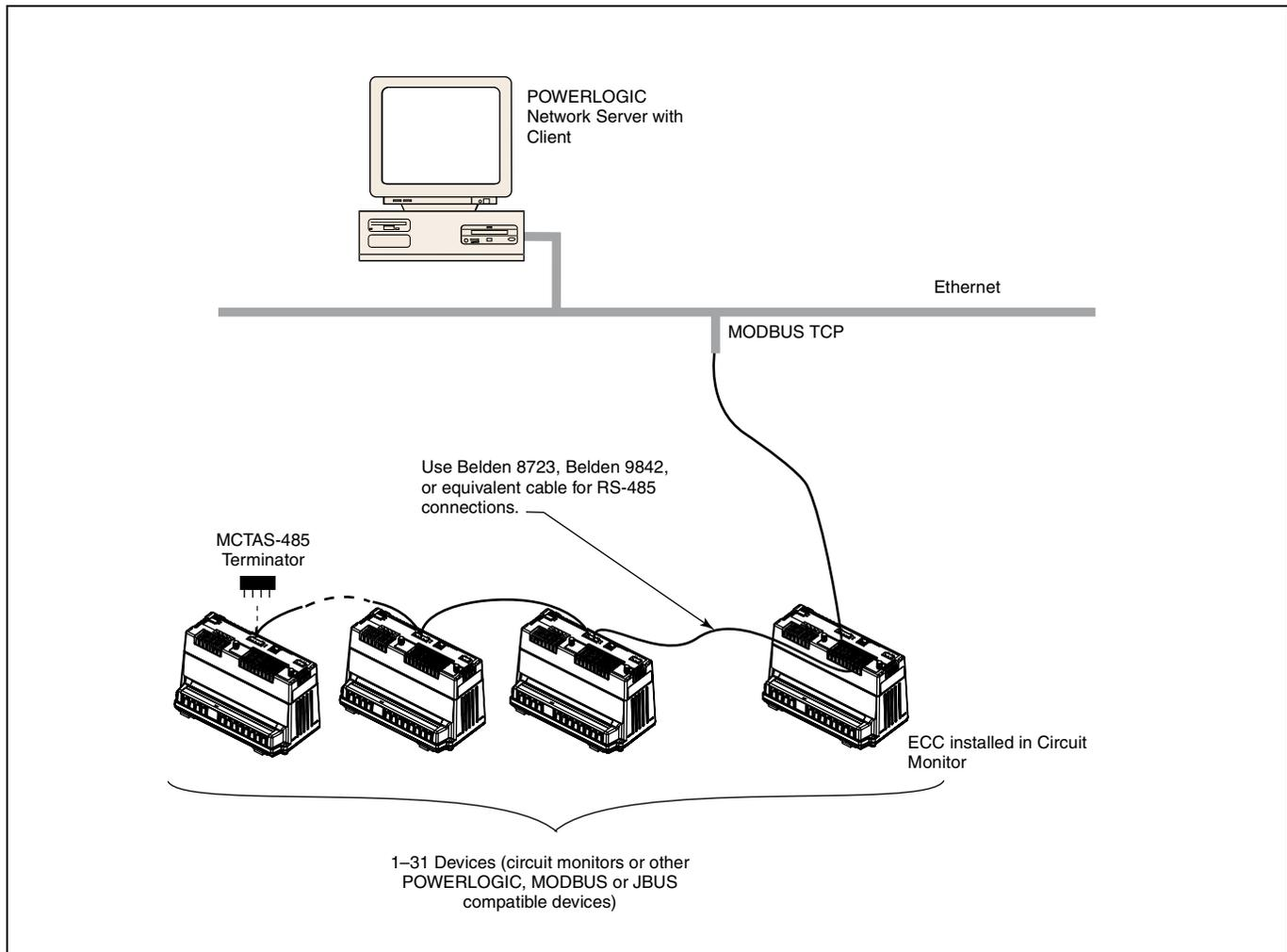
**Figure 6-13: Circuit monitors connected to an Ethernet Communication Card (ECC)**
