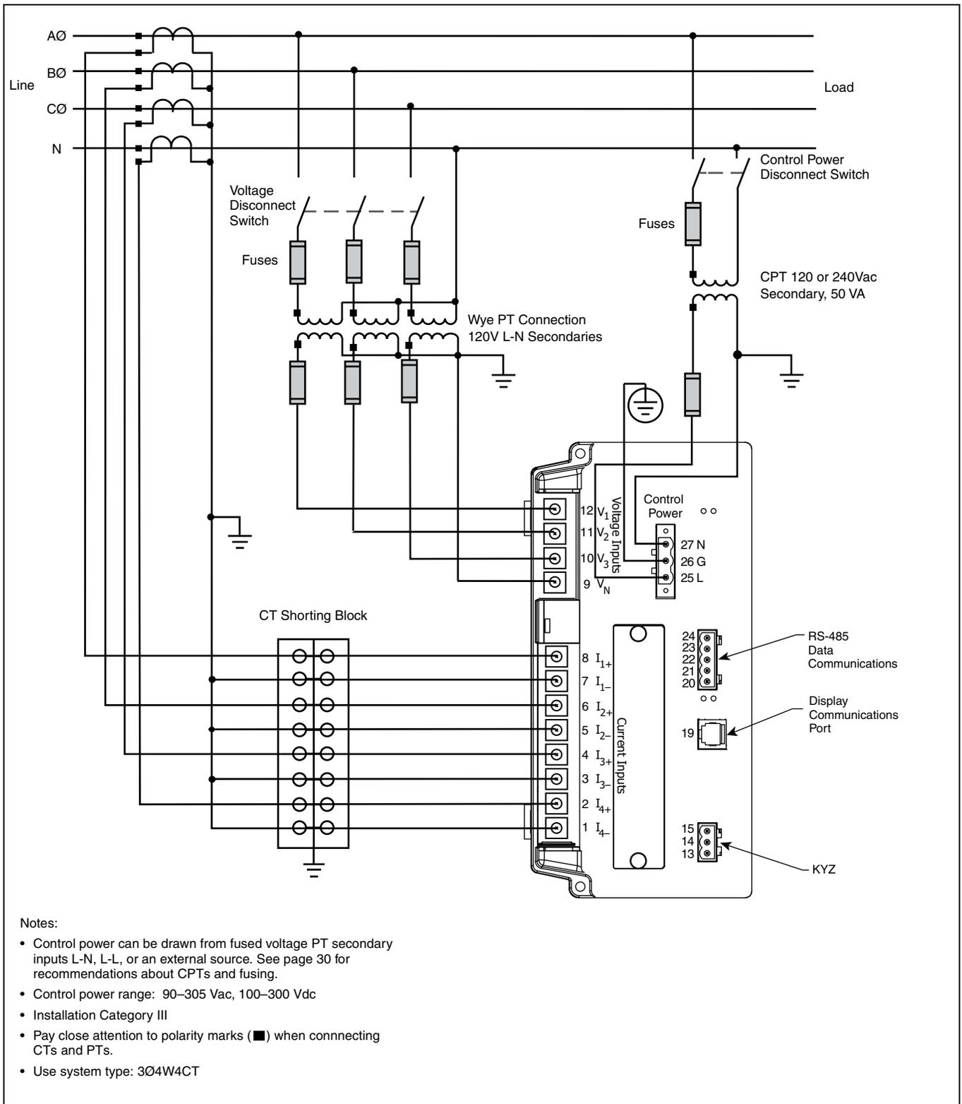
Figure 5–8: 3-Phase, 4-Wire Wye Ground Connection with 3 PTs and 4 CTs
