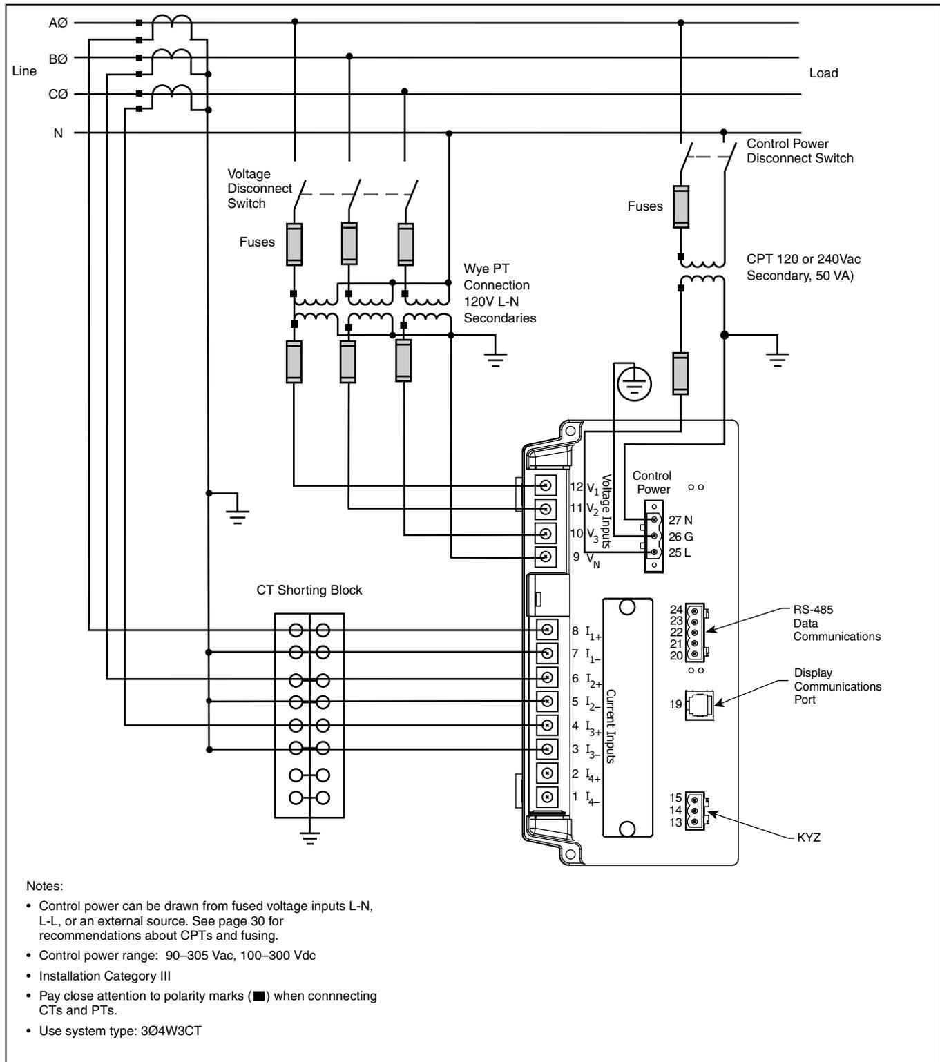
Figure 5–7: 3-Phase, 4-Wire Wye Ground with 3 PTs and 3CTs
