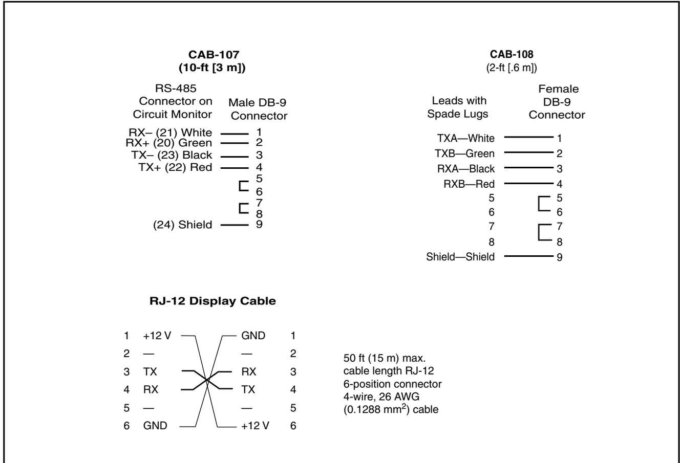
Figure B-1: Cable Pinouts
