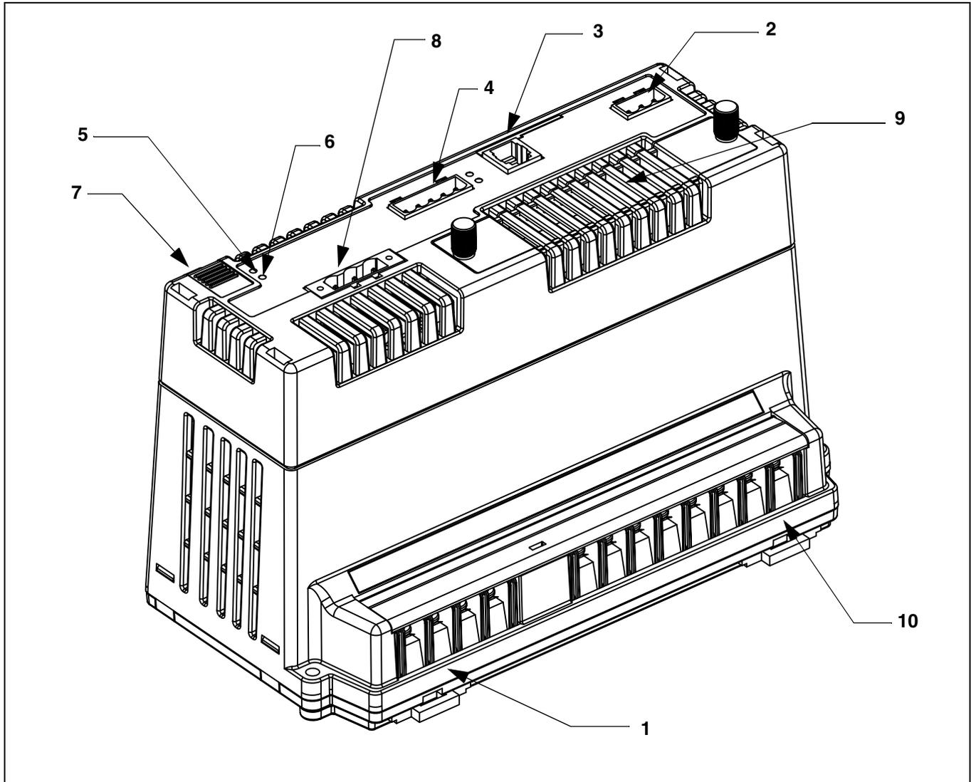
Figure 4-1: Parts of the Series 3000 Circuit Monitor
