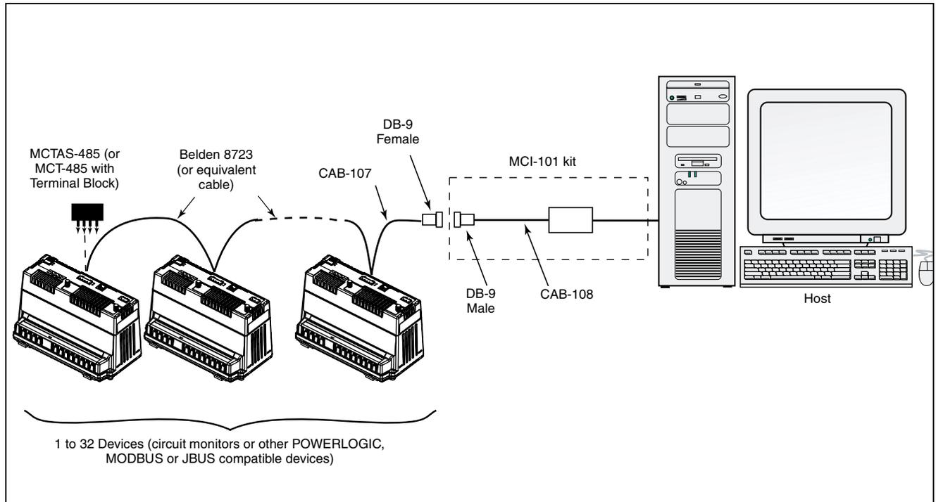
Figure 6–1: Circuit monitors connected to a PC serial port through the RS-485 port on the circuit monitor
