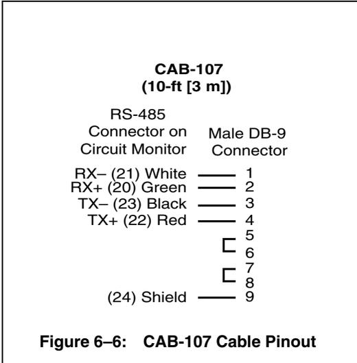
**Figure 6–6: CAB-107 Cable Pinout**
