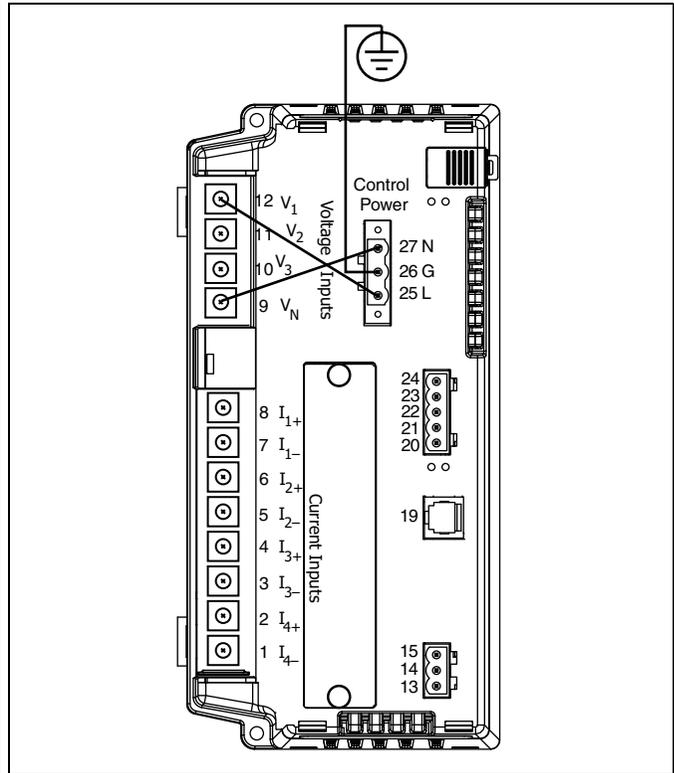
Figure 5-17: Deriving L-N control power from phase PT inputs (305 Vac maximum)
