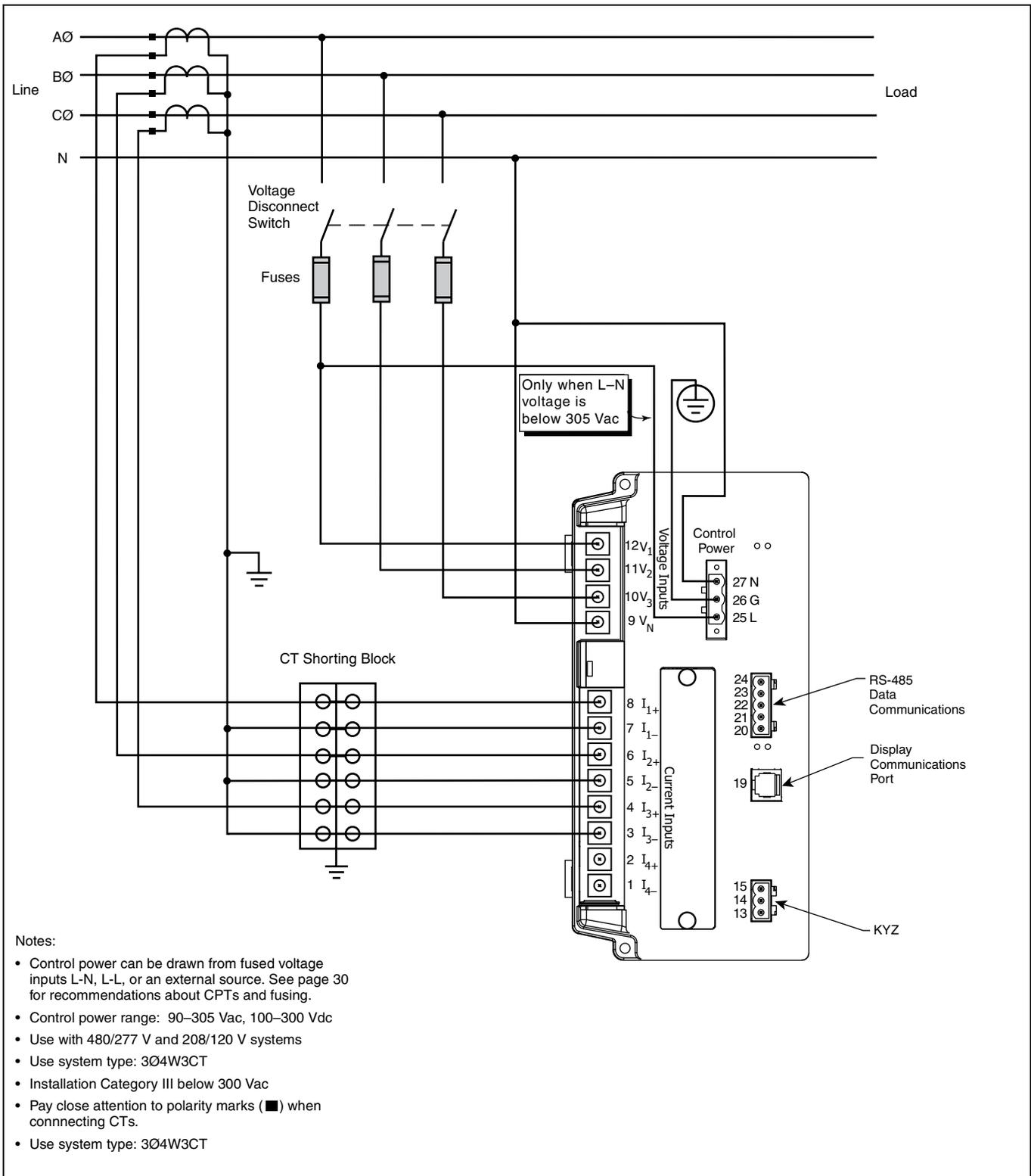
Figure 5–9: 3-Phase, 4-Wire Wye with Direct Voltage Connection and 3CTs
