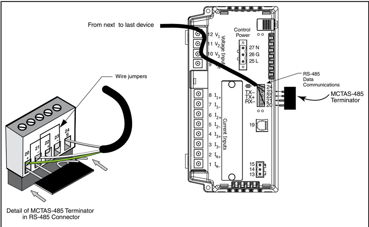
Figure 6–11: Terminating a circuit monitor wired for 2-wire MODBUS or JBUS communications
