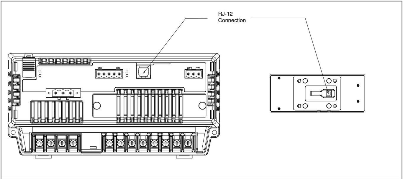
Figure 4-9: Display connection to the circuit monitor
