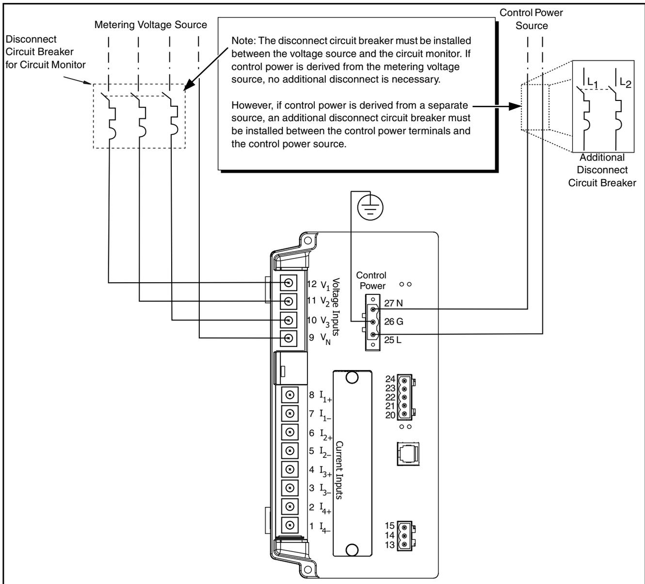
**Figure 5–3: Example of a disconnect breaker connection for CE compliance**
