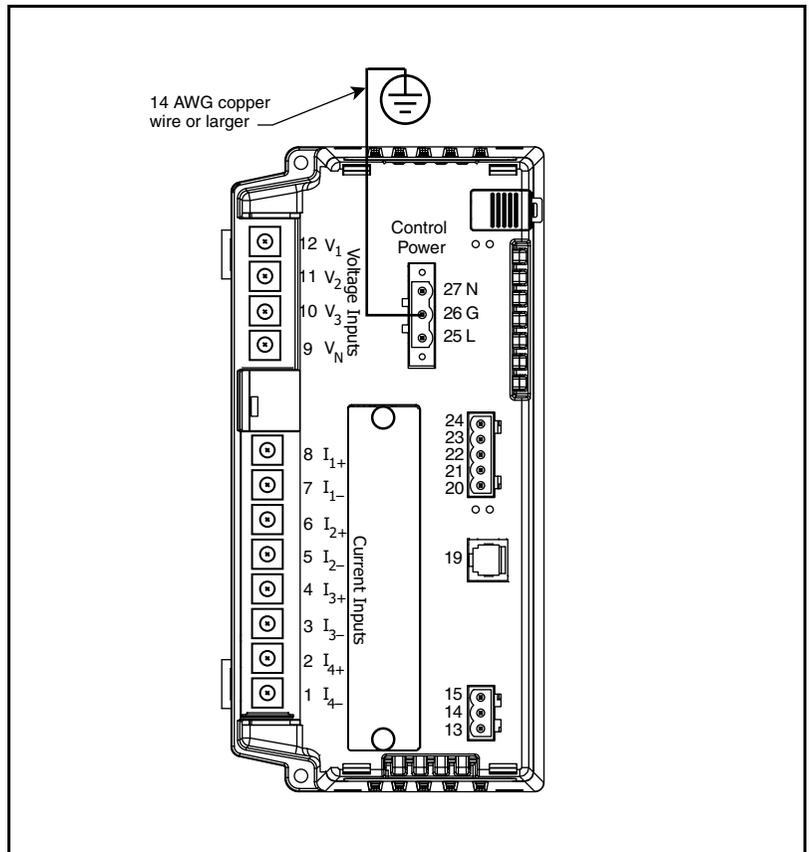
Figure 5–18: Connector for grounding the circuit monitor
