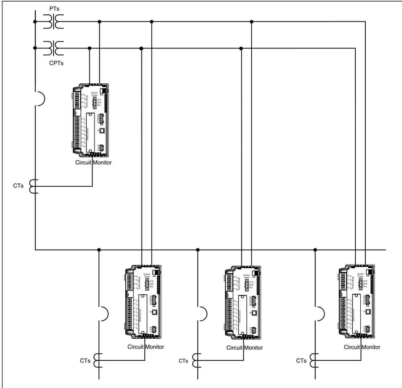
**Figure 5-15: Wiring multiple circuit monitors**
