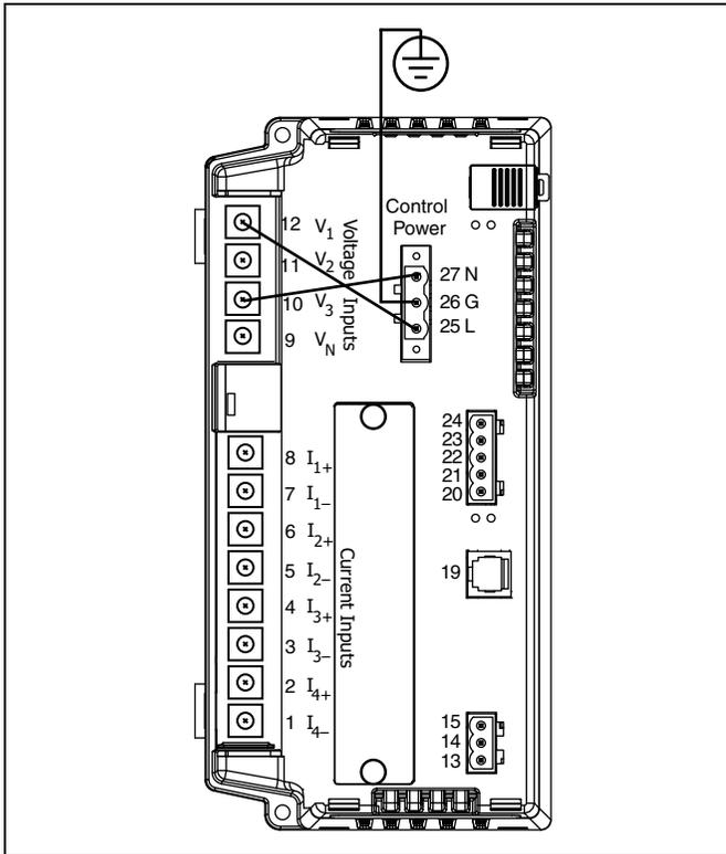
Figure 5-16: Deriving L-L control power from phase PT inputs (305 Vac maximum)
