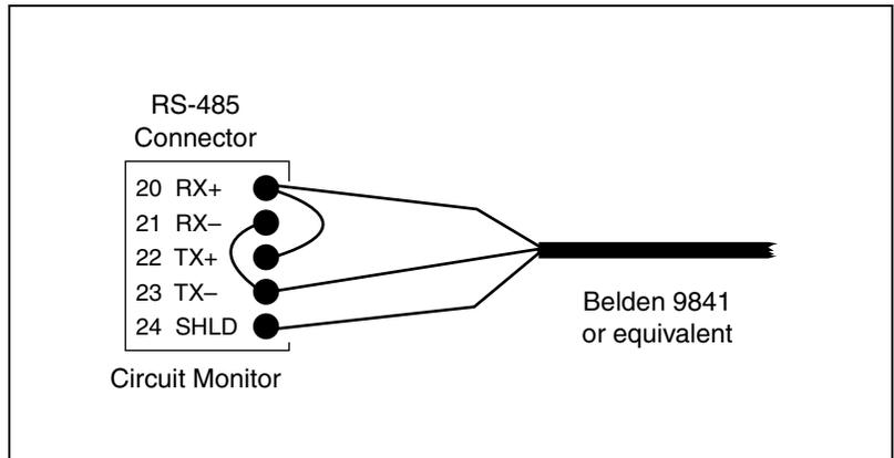
**Figure 6-10: 2-wire MODBUS or JBUS wiring**
