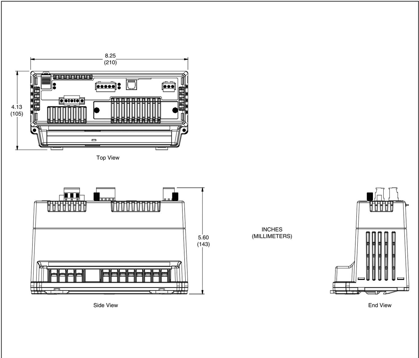
Figure 4-2: Circuit monitor dimensions
