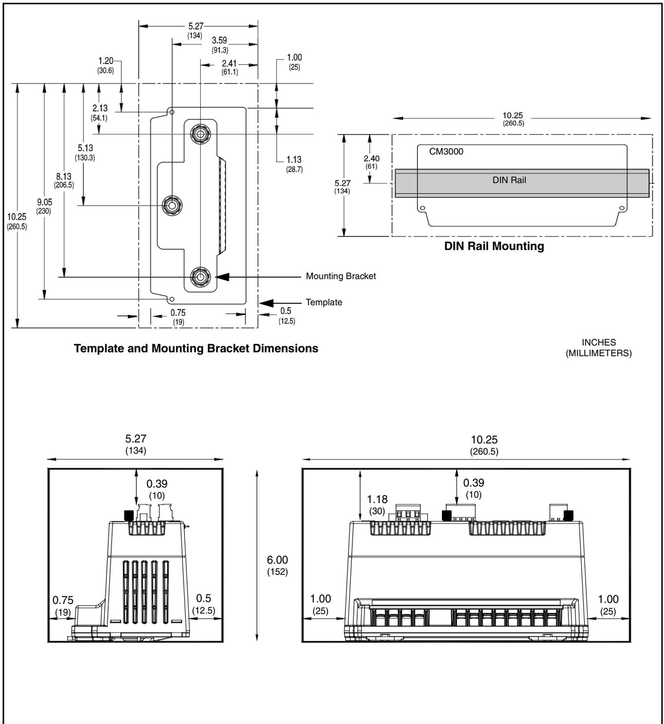
Figure 4-4: Dimensions and clearances
