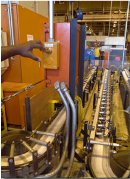
Line Operator Activates Pushbutton
