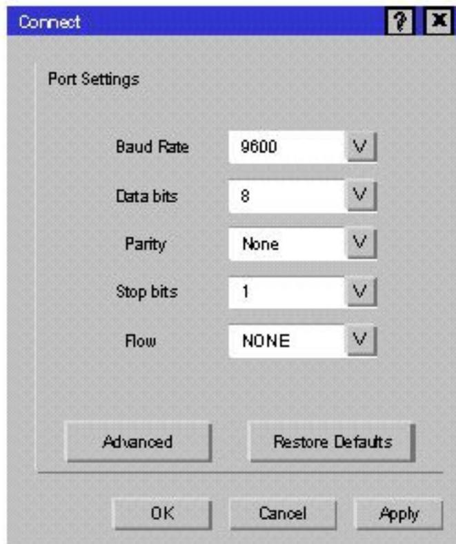
Figure 13 Example: RS-232 Serial Terminal Emulator Properties
