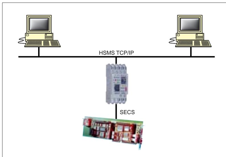
The bridge also allows multiple SECS networks to be linked together across an Ethernet connection. Multiple Bridges can furnish an Ethernet link between widely separated SECS networks. This extends the message path beyond the cable lengths allowed for serial connections,
