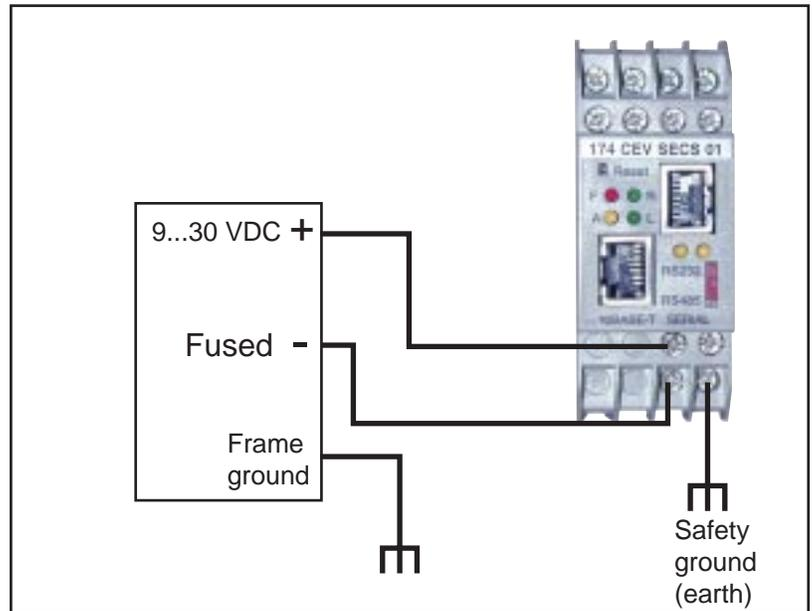
Figure 6 Connecting the Power Wiring
