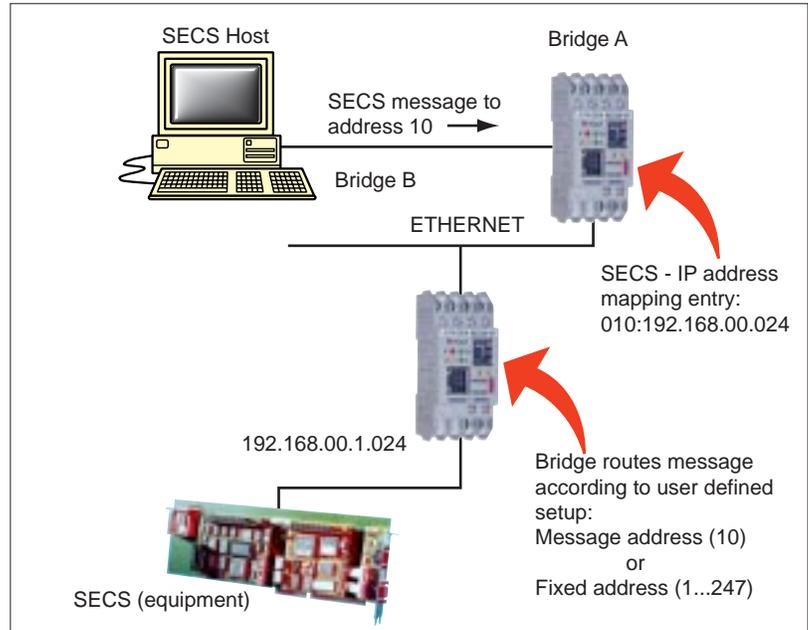
Figure 2 Bridging Between Multiple SECS Networks
