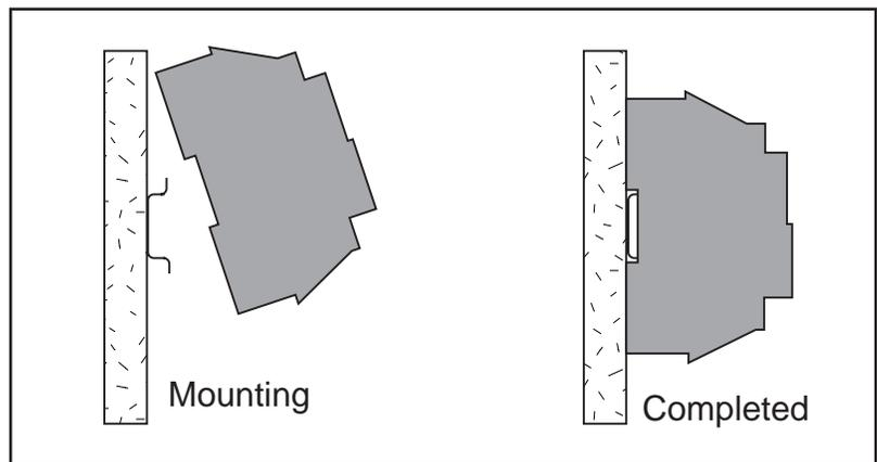
Figure 5 Mounting the Bridge on the DIN Rail
