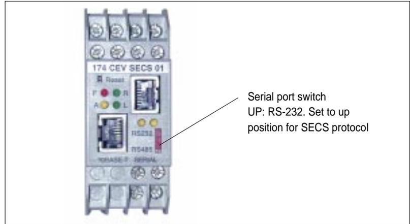
Figure 11 Setting the Serial Port Switch
