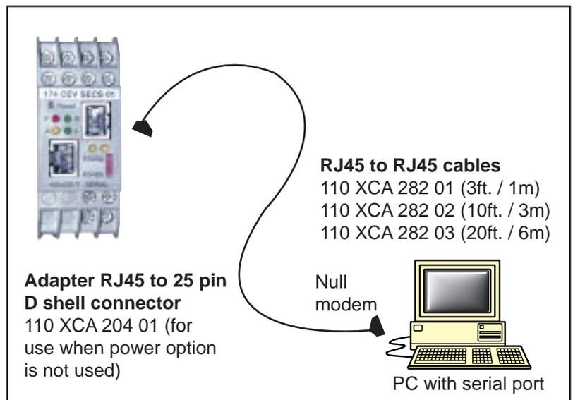
Figure 7 Connecting the Serial Cable (RJ45 Port)
