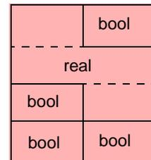
The real type member is considered as being stored on 3 addresses. The write would require 2 access bytes and 1 access word. When that is possible, it is preferable to build structures while taking into account the alignment criteria.
