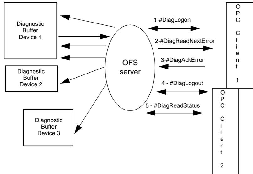
With the OFS server several PLCs can be monitored at the same time, it has a multi-station function (unlike the PL7 which can only manage one PLC at a time). To supervise several PLCs at once, simply create other aliases in the configuration tool and add them to another group belonging to the same client (minimum of 1 group per device to monitor).
