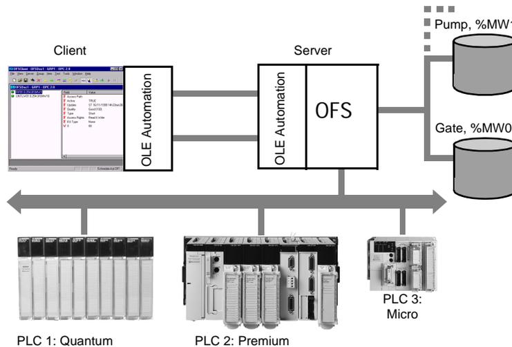
The OFS server provides the interface between devices and one or more client applications in which the values of some of the data of these devices are to be viewed and/or modified.
