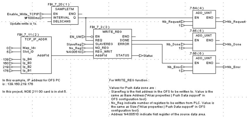
Some PL7 and Concept sample applications are provided on the CD to show how a PLC application can send Push Data to the server.
