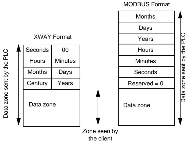
**Note:** With PL7, the date/time can easily be inserted using the RRTC function. With Modbus on Premium, if you are using RRTC, a BCD to INT conversion is required to match the Modbus format.
