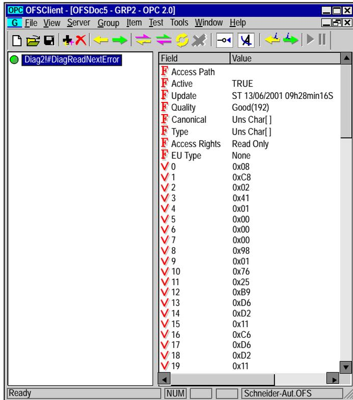
Example of translation of bytes V12 to V15 which represent the time of the beginning of the alarm. The table describing the time stamp format of the Diag buffer enables you to extract the different values.
