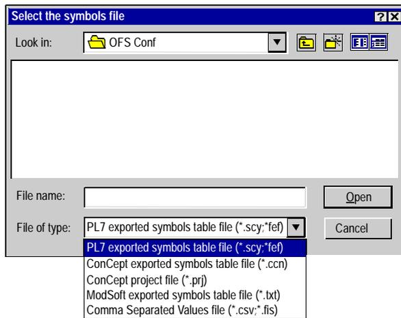
The file types that can be inserted are listed in the "type of files" list box. Select the appropriate file type.
