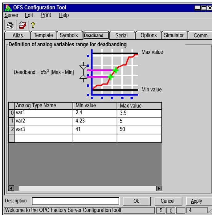
The range can be adjusted here for each variable, whether floating or integer, with minimum and maximum values.
