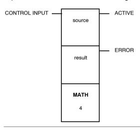
Parameter Description -Antilogarithm (base 10) Description of the instruction's parameters for the Antilogarithm (base 10) operation
