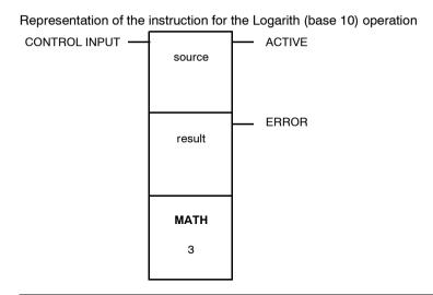
Parameter Description -Logarithm (base 10 logarithm) Description of the instruction's parameters for the Logarithm (base 10) operation
