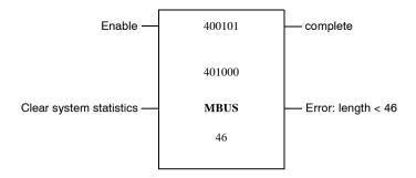
Register 400101 is the first register in the MBUS control block, making register 400103 the control register that defines the MBUS function code. By entering a value of 255 in register 400103, you implement a get statistics function. Registers 401000 ... 401045 are then filled with the system statistics.
