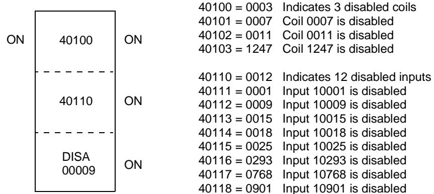
**Note:** The quantity of disabled discrete inputs is indicated as 12, whereas the allocated length for storage is only 9. This would indicate 4 additional disabled inputs exist for which insufficient 4XXXX storage space has been allocated. Since the inputs are listed in ascending numerical order those inputs not listed must be reference numbers greater than input number 1090 (the last one listed).
