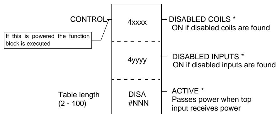
\*Note: All three outputs will be on regardless of the control input if the NSUP.EXE loadable is not available in the configuration.
