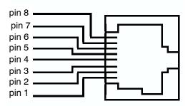
pins 3 and 6 provide one line pairpins 1 and 2 provide another line pairremaining pins are not used
