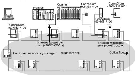
The following figure describes a Redundant Ring Structure.
