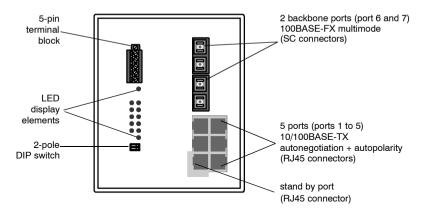
The following figure describes the interfaces, display elements, and controls of the ConneXium Switch 10/100 Mbps 7TX (499NES17100).
