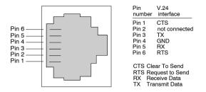
The socket casing is electrically connected to the front panel of the device.
