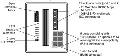
The following figure describes the interfaces, display elements, and controls of the ConneXium Switch 10/100 Mbps 7TX.
