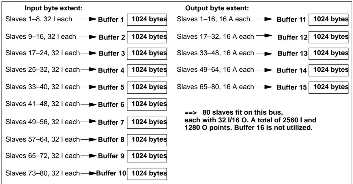
**Example of a scan of slaves with modular I/O for the large CPU (2)**
