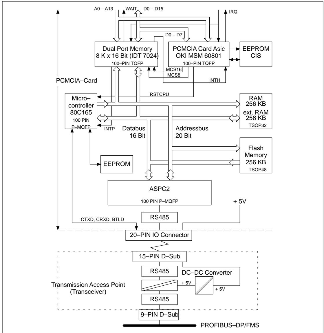
Figure 2 Functional Block Diagram of the PCMCIA Card + the Transmission Access Point
