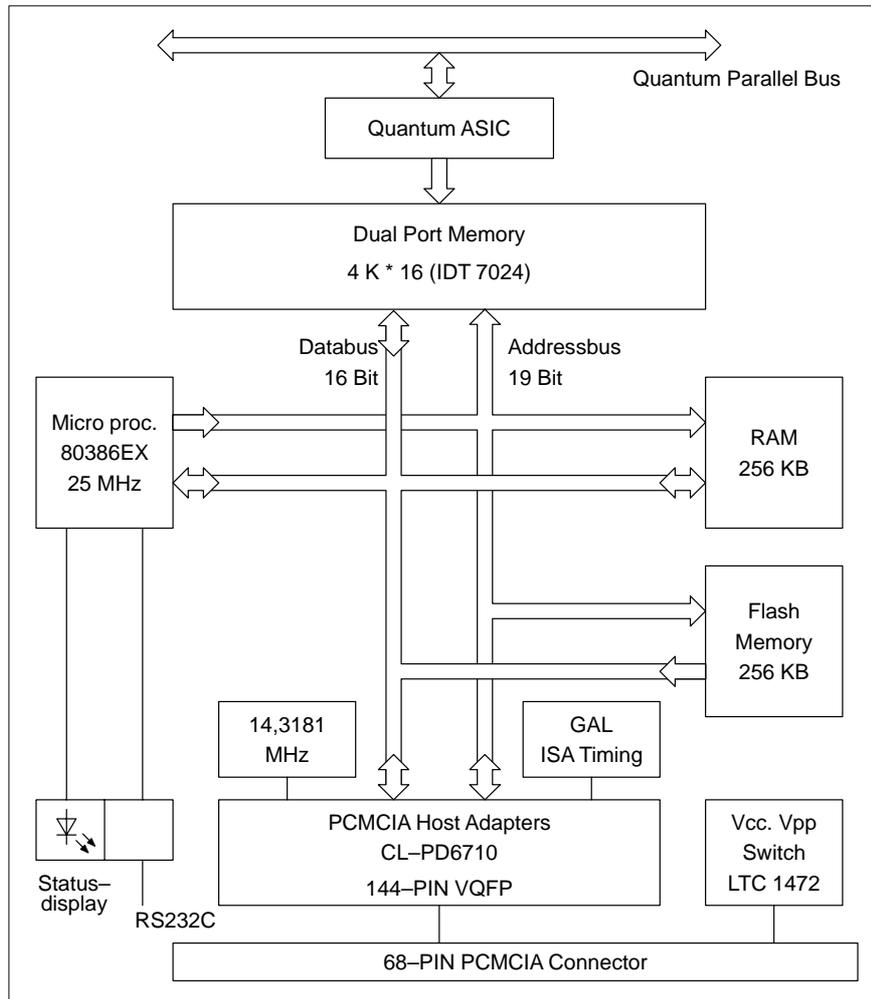
**Figure 1 Functional Block Diagram of the Quantum Module**
