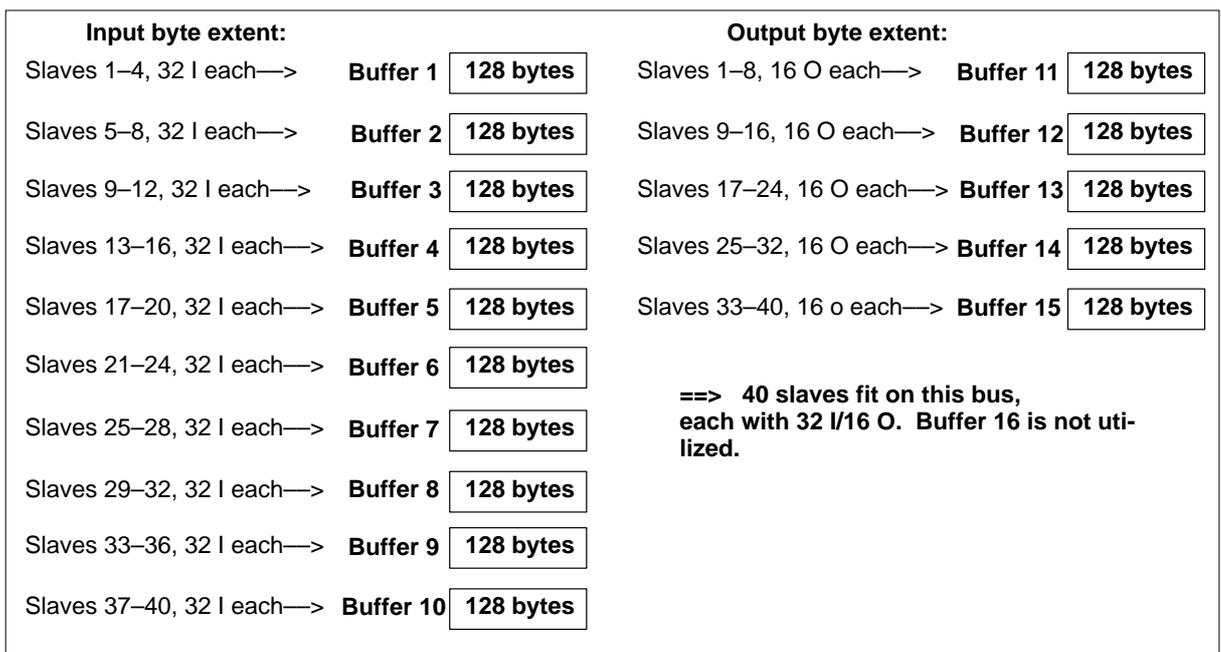
**Example of a scan of slaves with modular I/O for the small CPU (1)**
