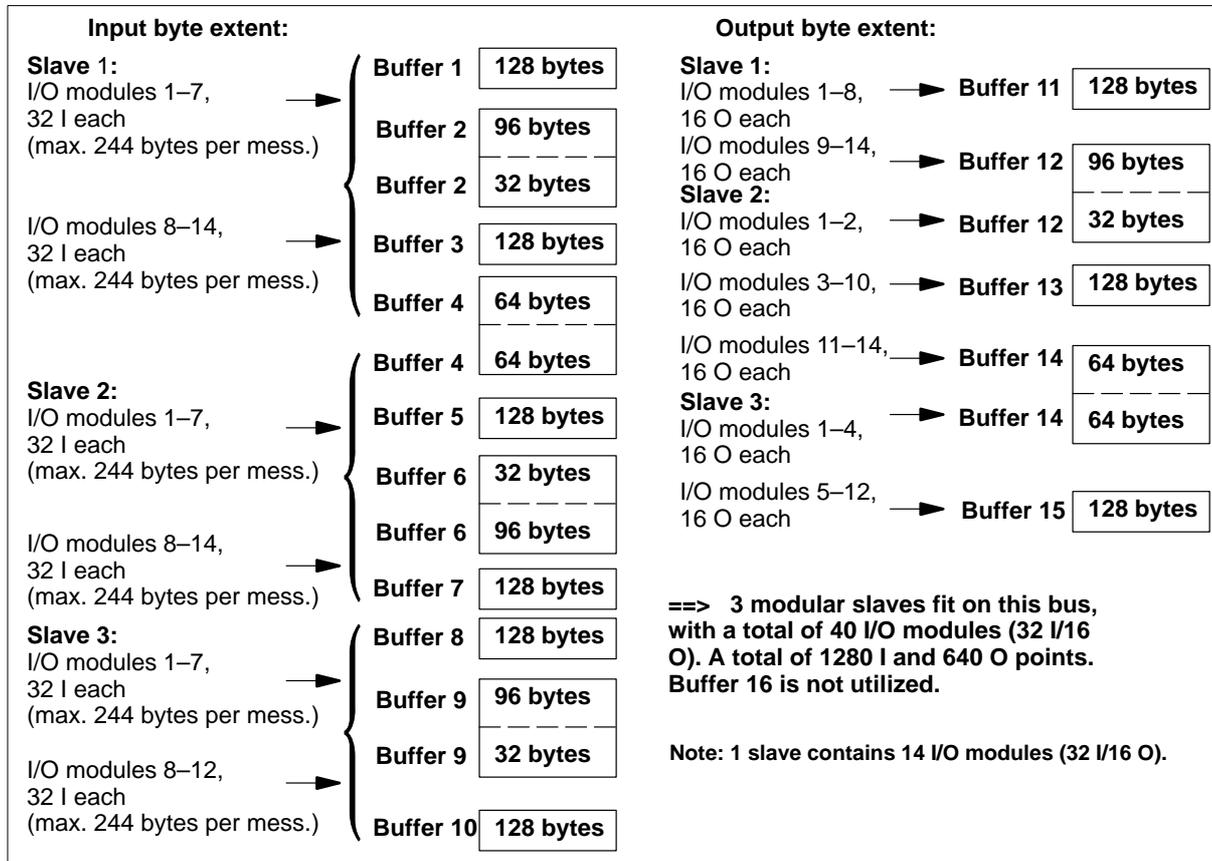
**Example of an I/O scan of Compact slaves with the large CPU (2)**
