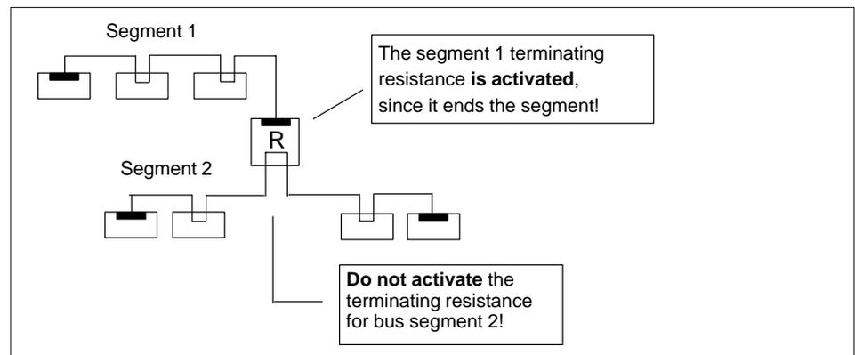
Only RS-485 repeaters of the IP 20 safety classification are allowed for rack installation (e.g., Siemens, order no. 6ES7 972-0AA00-0XA0)
