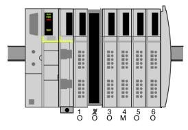
Suppose that the module in location 4 is mandatory and the optional module in location 2 is removed from its base, as shown below.
