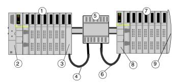
A preferred module can also pass the island bus communications signal to an extension segment of Advantys STB I/O modules, as shown below.
