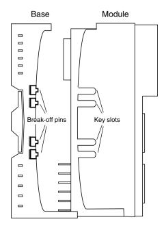
Here are the keying pattern combinations we will use to key our base/module combinations. The first six are unique. The seventh pattern is not.
