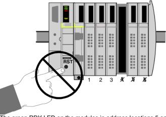
The green RDY LED on the modules in address locations 5 and 6 will flash to indicate that they are in pre-operational mode.
