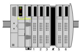
If you then place a new STB DDO 3230 output module in location 4, the NIM will recognize its device profile, configure it like the old module, and start supporting all six I/O modules the same as it did before the hot swap.
