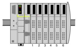
Suppose you have an STB DDO 3230 output module in address location 4, and it is malfunctioning. When you remove the module from its base, as shown below, the remaining five I/O modules in locations 1, 2, 3, 5 and 6 will continue to operate.
