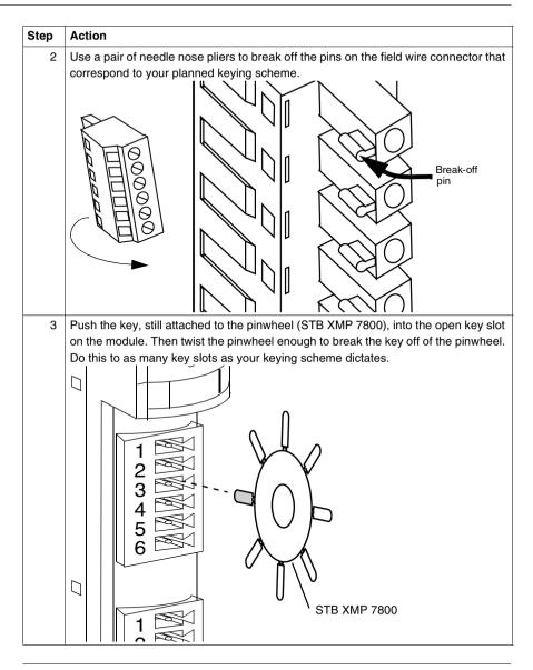
How to Key the NIM Power Connection The NIM power connector is a two-pin version of the I/O connector. Follow the same steps in *Keying the I/O Field Wire Connection* above.
