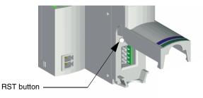
**Note:** Using the Advantys configuration software you can disable the reset button. In this situation pressing the reset button will not effect the existing configuration.
