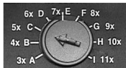
Figure 22: Circuit Breaker Trip Adjustment Dial
