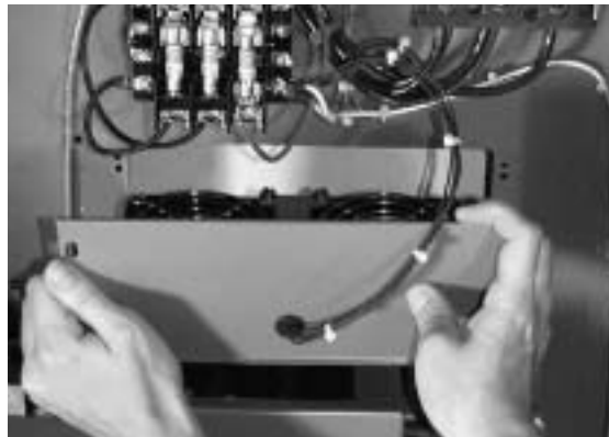
Figure 28: Remove the Heatsink Fan Assembly
