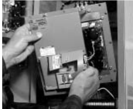
Figure 23: Remove Power Converter
