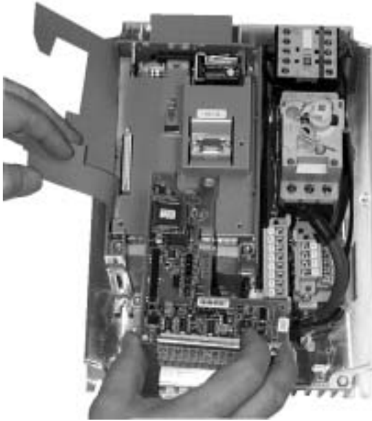
Figure 9: Installing an Option Card
